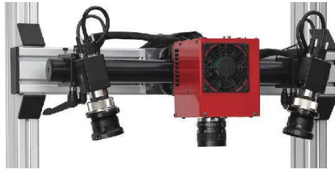
Figure 3: ARAMIS sensor with light source for FLC and bulge tests
